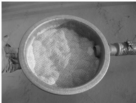
Fig. 5 Deep phosphine chamber – tablets spent and powder under mesh.
