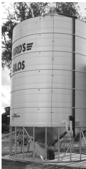
Fig. 1 Black thermosiphon pipe connected to reaction chamber at base
